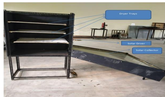
Figure 5: Complete Setup of Solar Dryer
