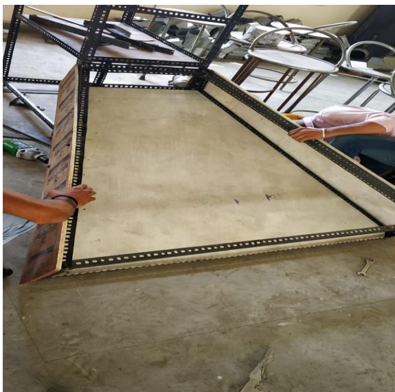
Figure 2: Wooden Planks Being Bolted with Collector Frame
